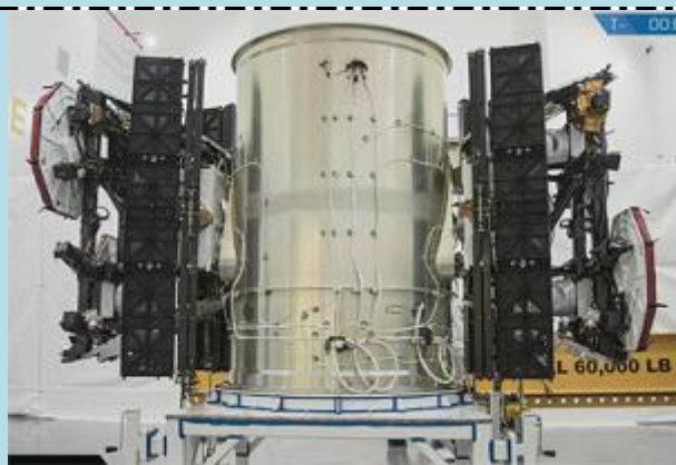
MicroSat 2a & 2B on adapter, 400 кг.
