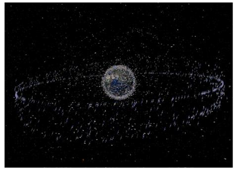
FIGURE 2.4.1 Artist's impression of the debris surrounding Earth. The number of objects in Earth orbit has increased steadily (by 200 per year on average) as more nations develop space programs. NOTE: Size of the debris greatly exaggerated as compared to the size of the Earth. SOURCE: Courtesy of the European Space Agency.
