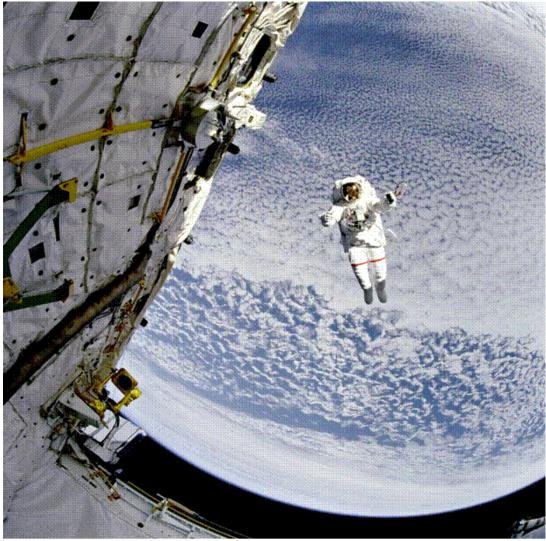
FIGURE 2.5 An astronaut tests the Simplified Aid for EVA Rescue system during an extravehicular activity. SOURCE: NASA.
