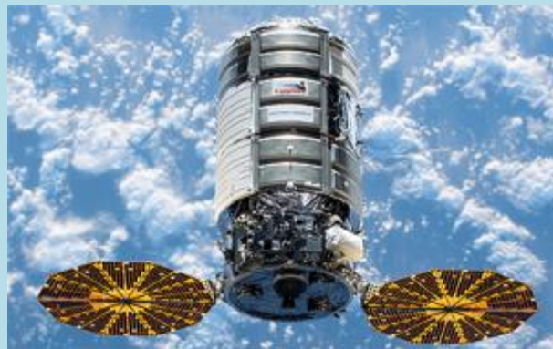
Cygnus CRS-12 (enhanced PCM version with radiators, external fittings and CubeSat deployers), 7492 кг.
