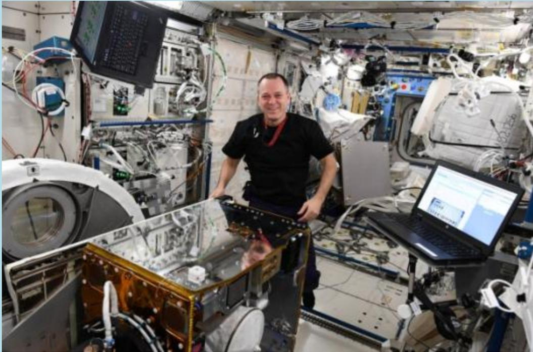
The RemoveDebris satellite, the largest ever deployed from the International Space Station, is moved into an airlock by NASA astronaut Ricky Arnold. It was deployed June 20, 2018.
